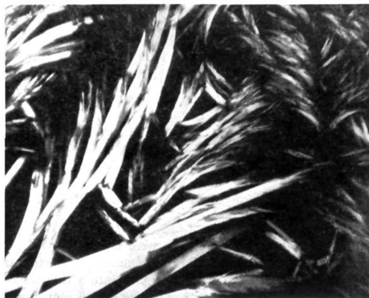
Fig. 3b.—Octadecylamine acetate in 95% ethanol; stable form, \times 200 .
